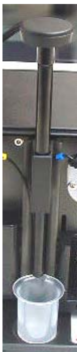
Figure 33: Injector carrier with injector in 'service position'.
