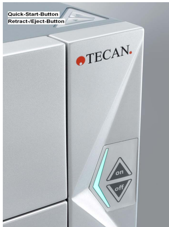
Figure 2: Onboard control buttons of Infinite M1000 . The ' Quick-Start-Script '-Button and the Retract-/Eject-Button are located in the front right corner of the top cover. The ' on/off '-button is located on the front of the instrument.
